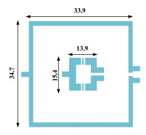
Figure 14. The layout comparison between proposed and typical WPD at 900 MHZ.
