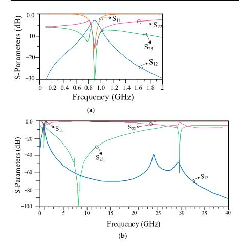
**Figure 11.** The scattering parameters at (**a**) operating band and (**b**) wide frequency range for the first design of the proposed WPD with 82% size reduction.
