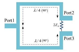
Figure 2. Microstrip realization of the typical WPD.
