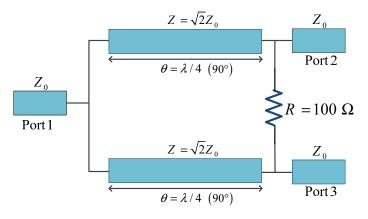
Figure 1. Schematic of a typical WPD.
