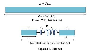
Figure 4. Structure of the typical and proposed developed branches.
