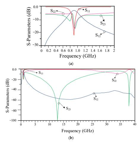
**Figure 13.** The scattering parameters at (**a**) operating band and (**b**) wide frequency range of the proposed WPD with 92% size reduction.
