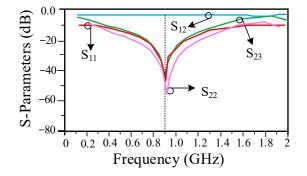
Figure 3. Frequency response of the typical WPD.
