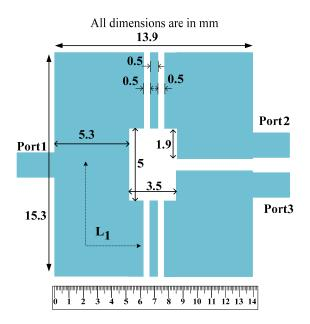
Figure 10. The first design of the proposed WPD at 900 MHz 82% size reduction.
