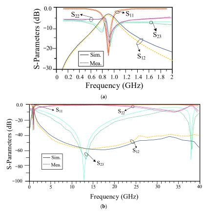
**Figure 16.** The simulation and measurement frequency response of the proposed WPD (**a**) at operating frequency (**b**) in the wide frequency range.
