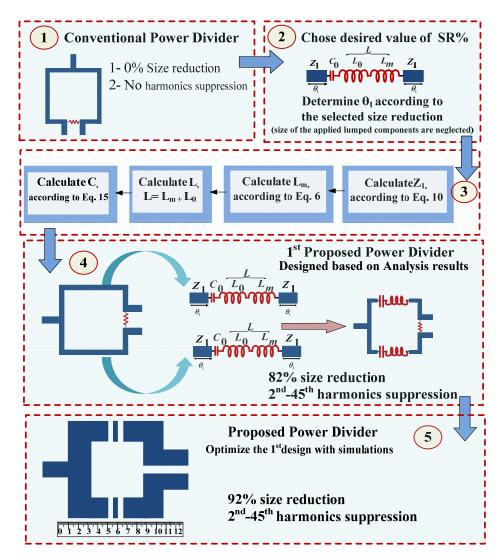
Figure 8. The design process of the proposed divider.
