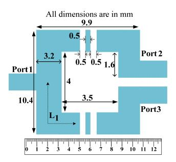
Figure 12. The proposed WPD at 900 MHz with a 92% size reduction.
