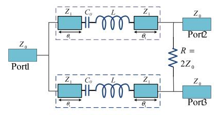
Figure 6. Structure of the proposed WPD with the series LC branches.
