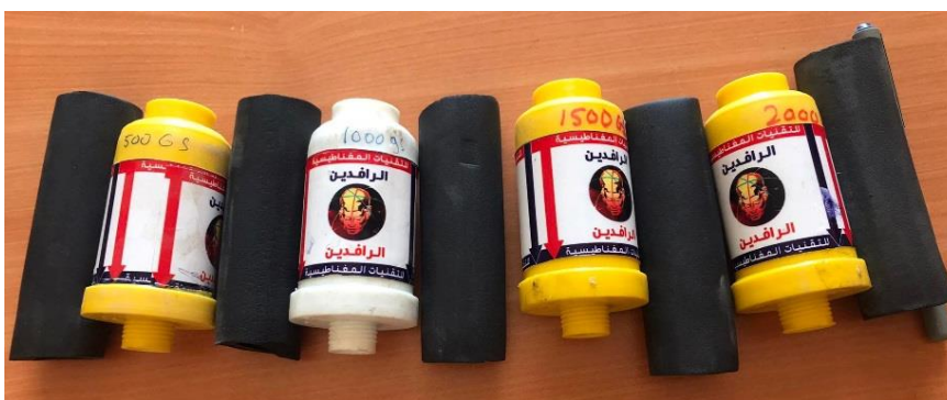
Figure 3.2. The Magnetic Devices Used to Magnetize the Study Waters
