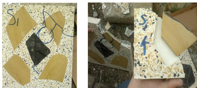
Fig. 10. Splitting failure of terrazzo tiles of factory (B).
