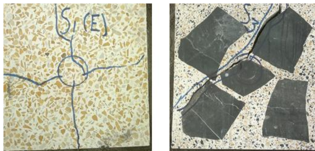
Fig. 9. Splitting failure of terrazzo tiles of factory (A).
